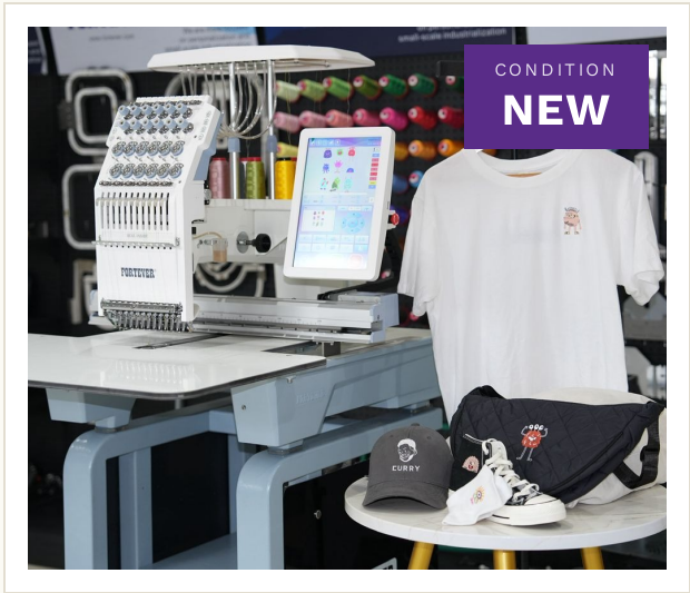
The CIRCUITSTITCH-15 — a single-head, 15-needle 360°-rotary platform for sampling embroidered circuits, antennas, and sensors.
