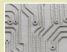
Conductive traces on woven substrate
